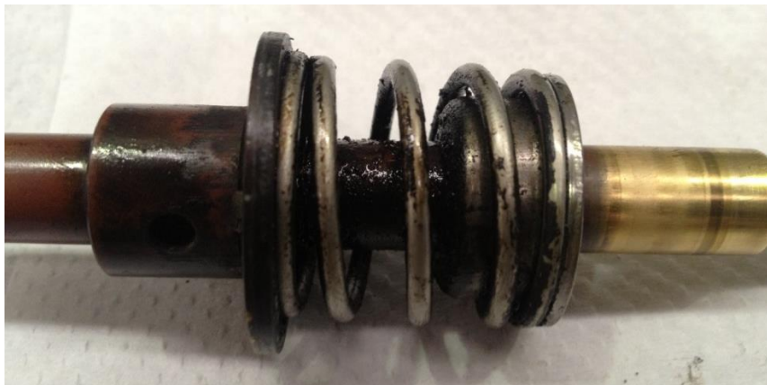
Figure 1: Contamination surrounding return spring
