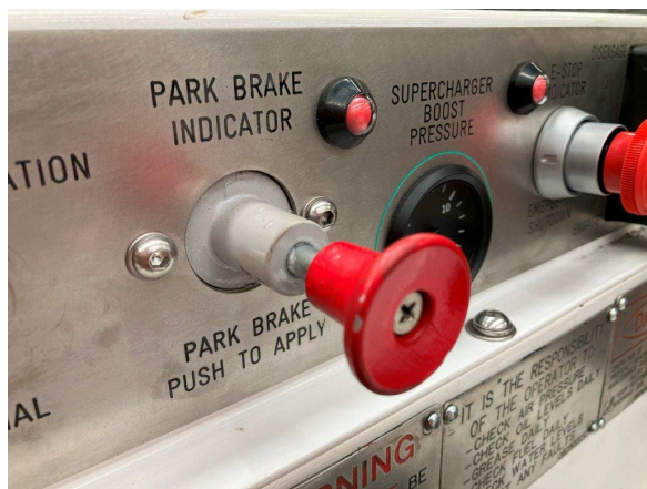
Figure 1. Original Park Brake Valve Installed shown from the operator's compartment. Note the 2 x mount bolts installed.
