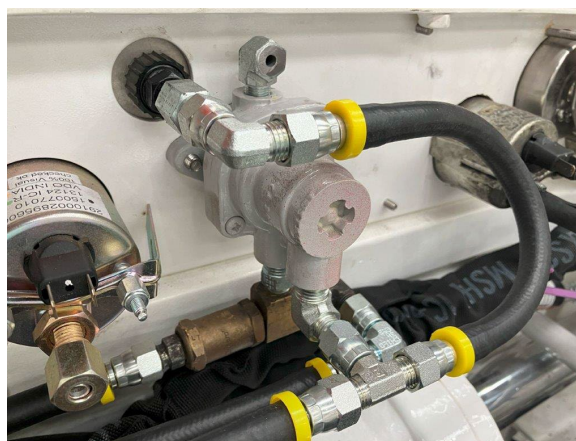
Figure 2. Original Park Brake valve viewed from the rear showing the hosing and fitting arrangement,
