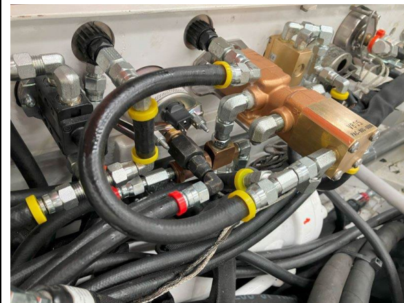
Figure 9. Park Brake valve viewed from the system delivery side showing the hosing arrangement.
