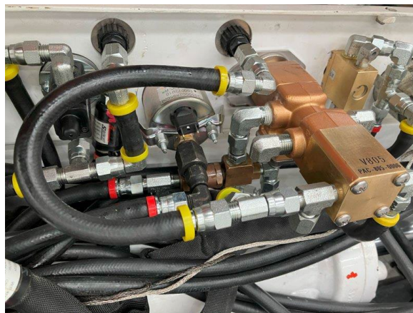
Figure 8. Park Brake valve viewed from the rear showing the hosing and fitting arrangement.
