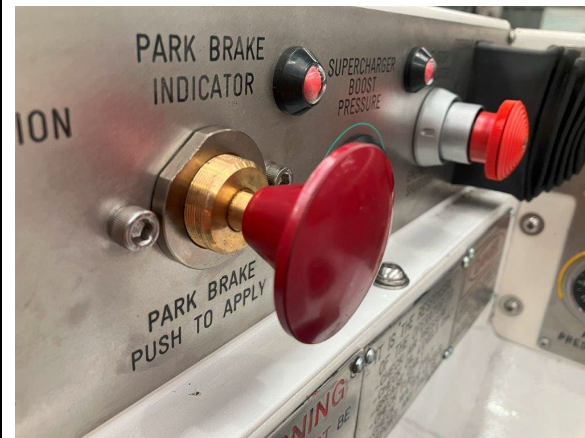
Figure 6. New Park Brake Valve Installed shown from the operator's compartment. Note the panel mount nut and 2 x mount bolts installed.
