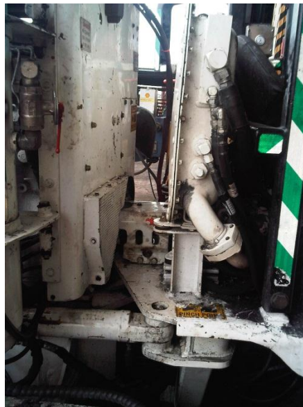
Area of Concern – Driveshaft Cover in Articulation
