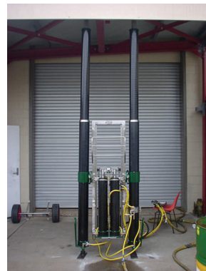
Pictured: High Seam Drill 2000, the two Stinger Legs allowing the drill to be rotated through 360°
