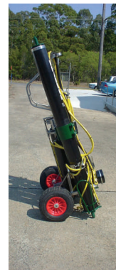
Pictured: High Seam Drill 2000, the two Stinger Legs allowing the drill to be rotated through 360°
