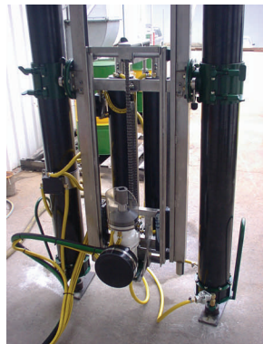
Pictured: High Seam Drill 2000, the two Stinger Legs allowing the drill to be rotated through 360°
