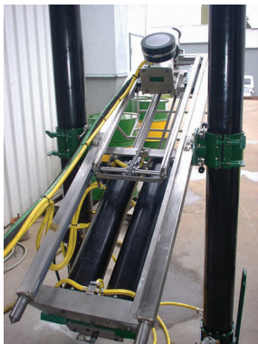
Pictured: High Seam Drill 2000, the two Stinger Legs allowing the drill to be rotated through 360°
